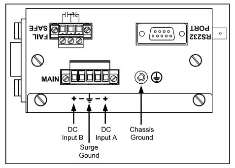
Figure 5 - DC Power supply wiring and grounding diagram
